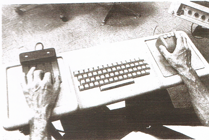
Inputs. Conventional keyboard is in parallel with 5-key handset, whose combinations correspond to individual keys. At user's right hand is a "mouse," the movements of which on any smooth surface are duplicated by a spot, or "bug," on the display. Shown inverted at left, the mouse has two wheels and a ball bearing for three-point support.
