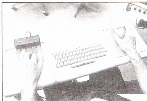
Overhead view of the "all in one" Console showing the Keyset, Keyboard and Mouse
